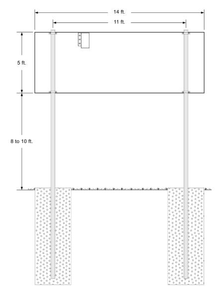
Once you have verified the positions of the posts and the size of the footings, you are ready to dig your holes, pour your concrete, and set your posts. There are several techniques for ensuring proper alignment of the posts. Typically installers will construct a temporary wooden support frame to hold each post in place while the concrete sets. Having plumb posts in the proper position is the key to a smooth mechanical installation.
